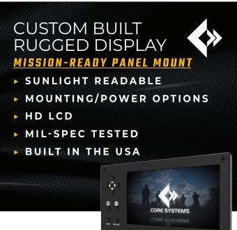
The rugged MPM7 is shock mounted and has been tested to meet DO-160E standards. Our LCDs go under rigorous MIL-Spec testing to ensure the highest quality ensuring the MPM7's ability to thrive in a variety of applications on the ground, in the air and out at sea.
